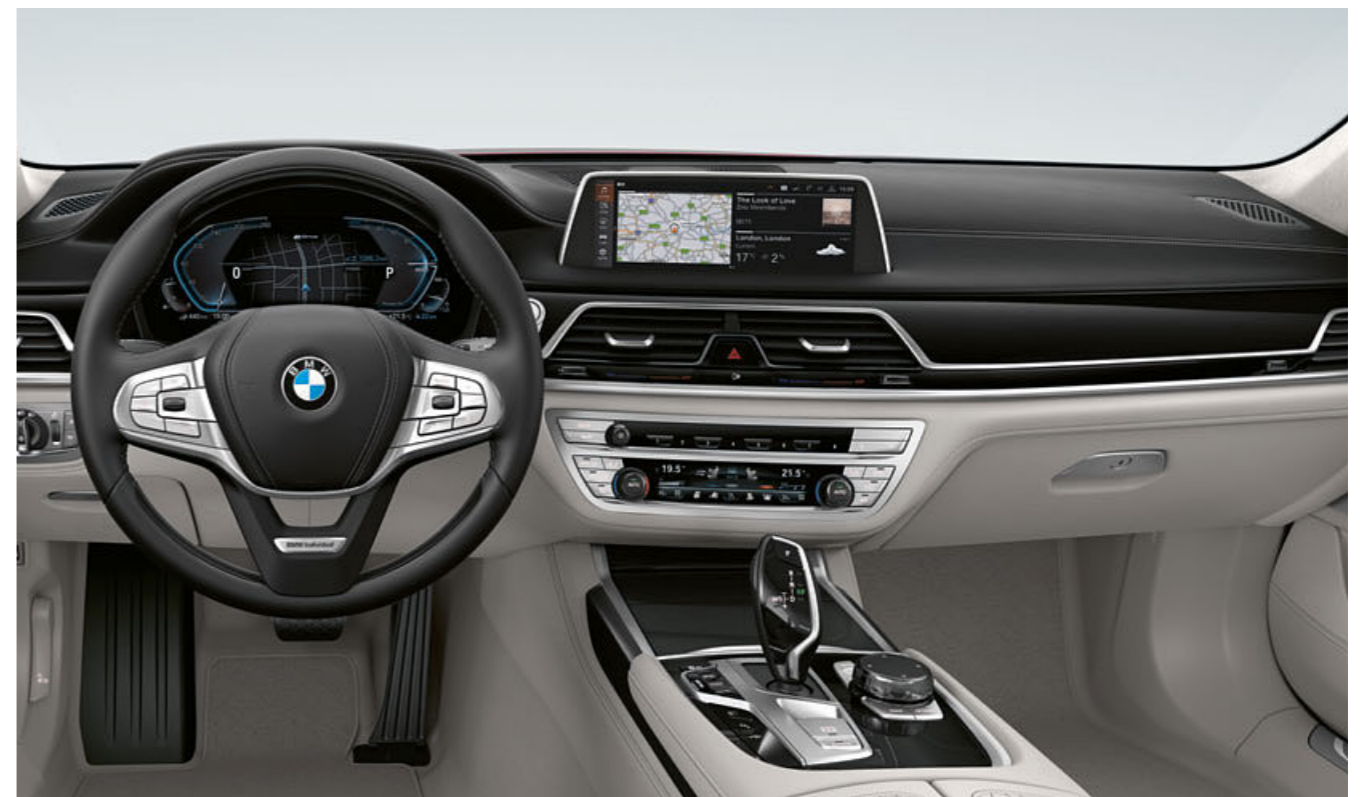
THE BMW INDIVIDUAL INTERIOR TRIM FINISHERS PIANO FINISH BLACK ARE APPLIED AND POLISHED ON A BLACK COLOURED TULIP WOOD VENEER IN SEVERAL LAYERS OF CLEAR PAINTWORK, UNTIL THE CHARACTERISTIC DEEP HIGH-GLOSS EFFECT IS ACHIEVED.
