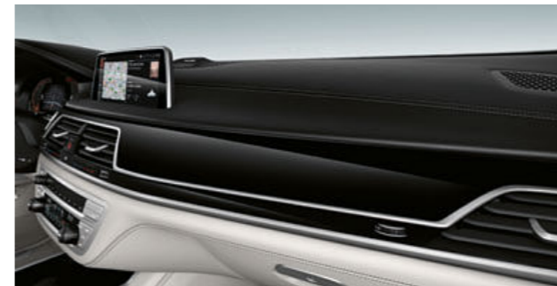
THE BMW INDIVIDUAL INTERIOR TRIM FINISHERS PIANO FINISH BLACK ARE APPLIED AND POLISHED ON A BLACK COLOURED TULIP WOOD VENEER IN SEVERAL LAYERS OF CLEAR PAINTWORK, UNTIL THE CHARACTERISTIC DEEP HIGH-GLOSS EFFECT IS ACHIEVED.
